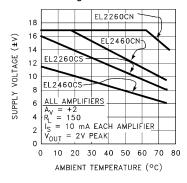
The curves do not include heat removal or forcing air, or the simple fact that the package will probably be attached to a circuit board, which can also provide some form of heat removal. Larger temperature and voltage ranges are possible with heat removal and forcing air past the part.
